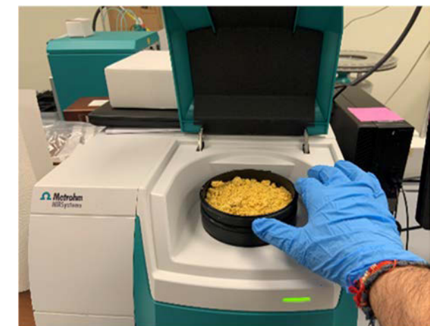
Figure 1. Fermentation mash sample placed on the DS2500 Solid Analyzer.
