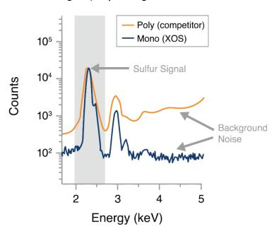
Figure 4: Superior Signal-to-Noise Ratio
