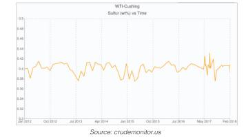
Figure 1: Sulfur Content of WTI Delivered at Cushing
