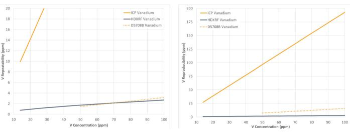
The results of this study show that Petra MAX, powered by HDXRF, is more efficient and delivers precision comparable or better than the ICP ASTM test method precision (D5708B) for nickel and vanadium in crude oil.
