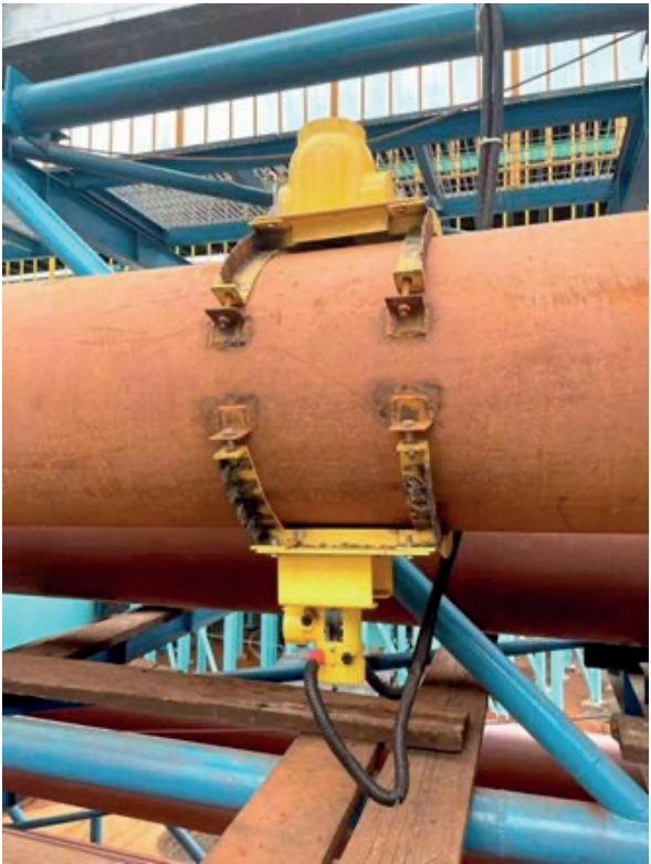
VEGA MINITRAC 31 performing radiometric density measurement in a pipeline
