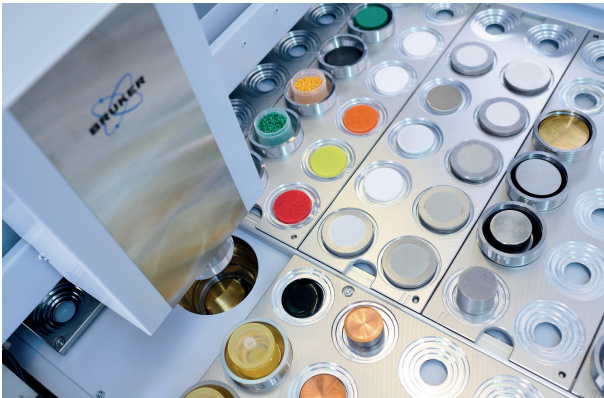
Figure 2: Innovative EasyLoad™ magazine accommodates various sample types in a single design.
