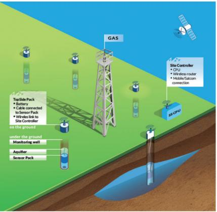
Figure 1: visualisation of ShaleSafe technology deployed in the vicinity of a shale gas well site.
