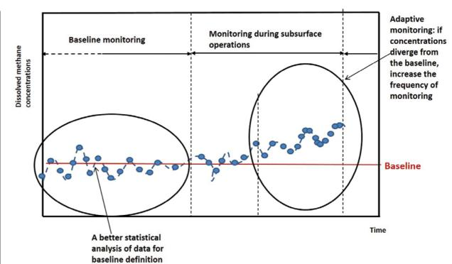
Figure 2: how better evaluation of trends can be obtained using ShaleSafe
