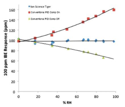
Figure 4: Effect of humidity on the response of a conventional 2-electrode PID and a humidity resistant PID.
