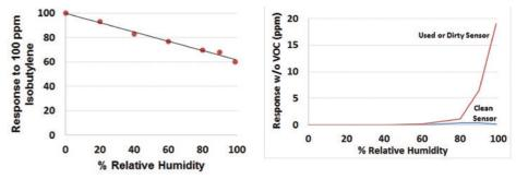
Figure 2: Left. Quenching of VOC response at high RH. Right Drifting reading in clean air at high RH.
