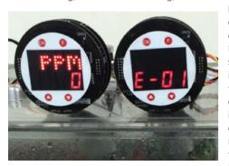
Figure 5: Fixed PIDs a) with (left) and b) without (right) condensation control
