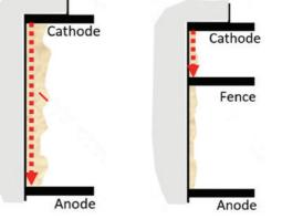
Figure 3: Leakage current at high humidity is trapped in the fence-electrode system.
