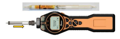
Figure 7: Pre-filter tube attached to PID for specific benzene measurements in a portable instrument.
