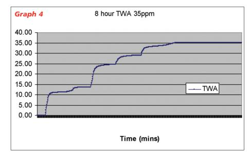
pattern. Most personal gas detectors take this into account and will continue to calculate cumulative exposure using 480 minutes rather than 720 minutes.
