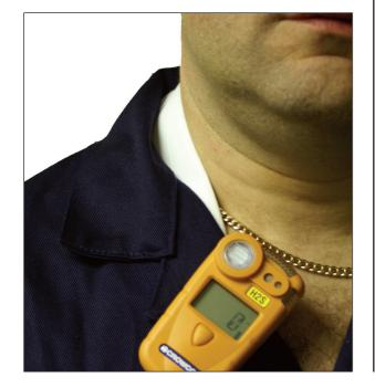
As you might expect, the LTEL for any toxic gas is a lower value than the STEL. For example, hydrogen sulphide has a STEL of 10ppm and an LTEL of 5ppm, reflecting the importance that both long and short term exposures are considered during any working period.
