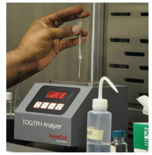
produced water is within the accepted limit required to pump overboard. The same technology is ideal for testing the wastewater from hydraulic fracturing as the analysis does not require a skilled laboratory technician and can be done on-site in less than 15 minutes-reducing the cost and delay of laboratory analysis.
