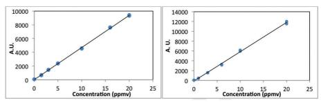
Figure 2: Hydrogen sulphide in nitrogen (left); total sulphur content using COS in nitrogen (right).
