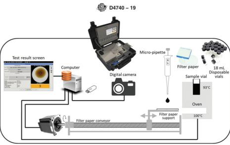
Figure 2. Schematics of the automated apparatus (Source : ASTM [1])
