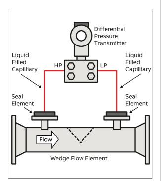
By mounting the installation horizontally, liquids, solids and entrained air are able to pass freely through the wedge restriction, in contrast to conventional orifice plate technology, where process material can build up on the measurement face, resulting in a 'damming' effect.
