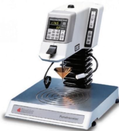
Figure 3: Digital Penetrometer [13].
