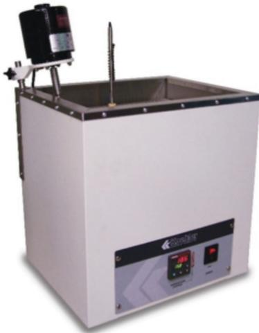
Figure 2: Copper Strip Corrosion for Lubricating Greases
