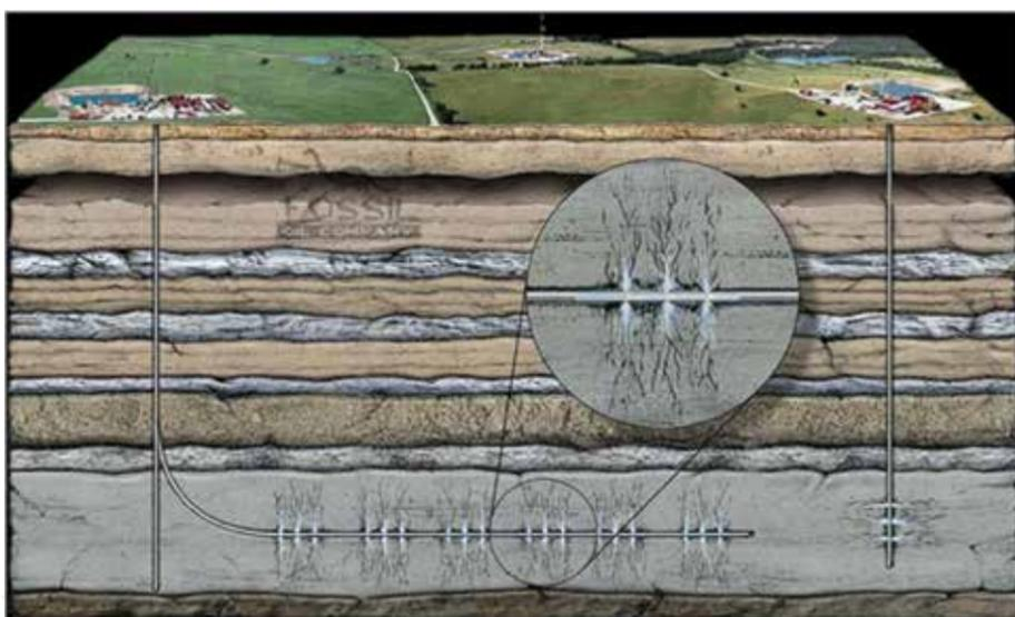
Figure 2: The Horizontal Well compared to a Vertical Well
