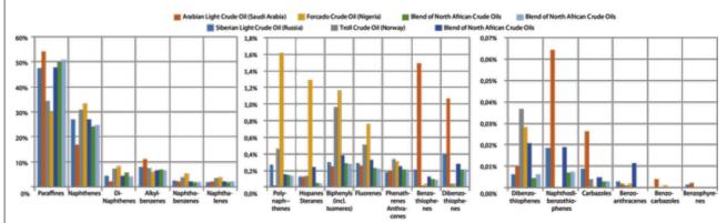
Figure 3: Comparison of different crude oils and blend based on a detailed chemical analysis obtained by GCxGC-TOFMS. The assignment to the compound classes was confirmed by accurate information obtained by high-resolution time-of-flight mass spectrometry.
