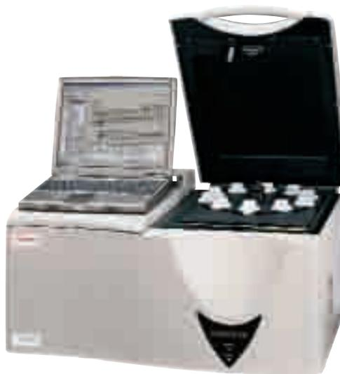
for chlorine. Calibration was performed in the range of 5 to 1000 ppm. To reach an acceptable compromise between acquisition time and limit of detection two excitation conditions were required with a time of 7 minutes per condition. This is possible thanks to the close coupling distances: tube-sample-detector that a direct excitation system like the ARL QUANT'X can provide.
