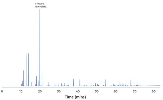
Figure 2. Front end analysis of crude oil sample to ASTM D7900 specifications
