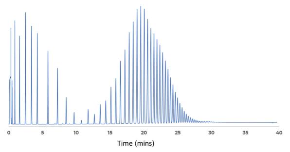
Figure 1. Chromatogram of D7169 calibration standard ( $C_5$ - $C_{100}$ )
