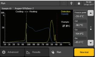
FIGURE 3 shows a typical freezing point graph for jet fuel on an OptiFZP. The difference between the coldest temperature which crystals are formed and the freezing point is 6.4°C.
