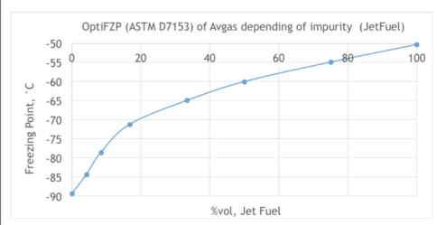
The graph in FIGURE 2 shows that low levels of jet fuel contaminating Avgas can be detected with the OptiFZP because the instrument can go to very low temperatures and the two-detector detection system picks up both large and small crystals.
