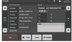
What meaningfully affects the Avgas freezing point are components that significantly varies from the petroleum alkylates used in today's blends. One example is the effect on freezing point temperature of Avgas contaminated with jet fuel. A customer had a real-life issue with jet fuel contaminating his Avgas. In order to determine effect of jet fuel contamination on freezing point, the customer dosed his Avgas with Jet A-1.
