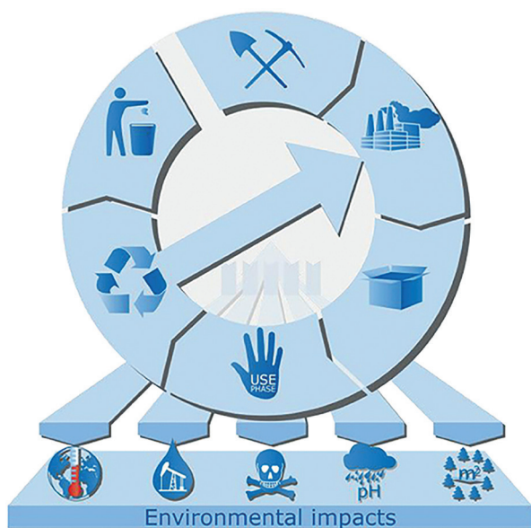
Figure 2: The holistic approach of life cycle assessment accounts for environmental impacts associated over the entire life cycle with all stages of product's life cycle (circle in the middle) [7].
