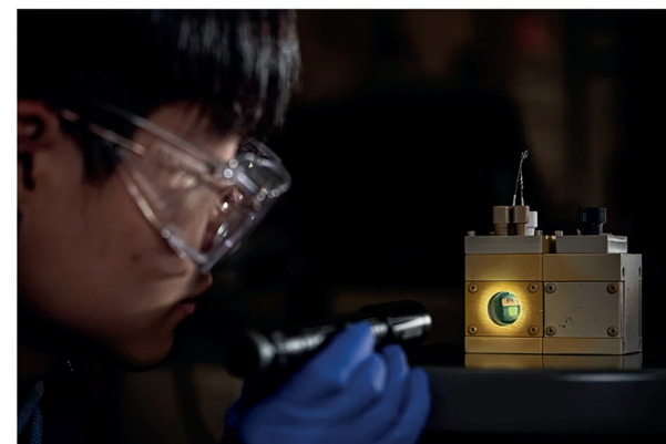
Figure 14: The Berkeley Lab postage stamp sized artificial leaf device [26].
