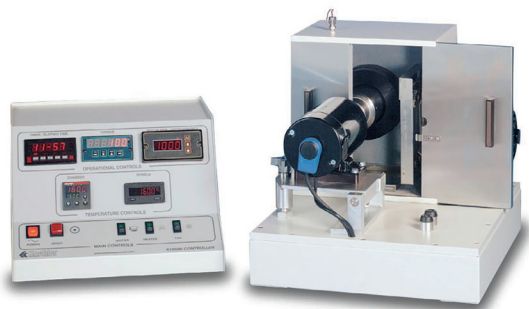
Figure 7: High temperature wheel bearing grease tester. Conforms to ASTM D3527, D4290 and D4950.
