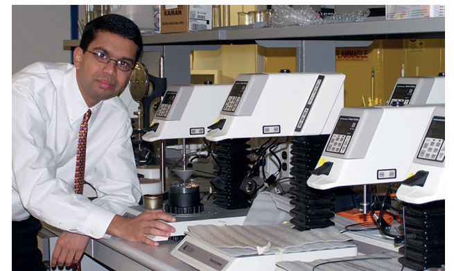
Figure 2. Penetrometer with a penetration cone: Conforms to ASTM and related specifications for penetrometers.
