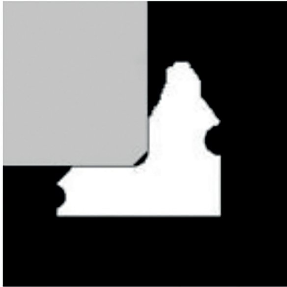
Figure 2a. Marginally Acceptable Electrode Edge[6]
