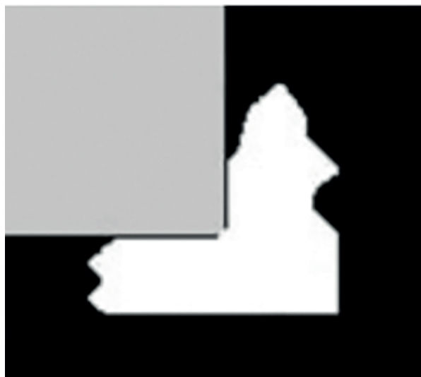
Figure 2b. Unacceptable Electrode Edge[6]
