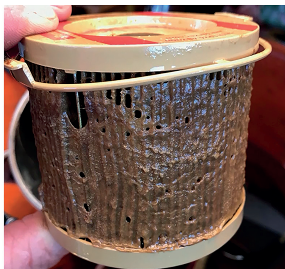
Figure 6: Carboxylic acid deposits in a fuel filter [8]
