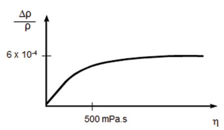
Figure 5: Viscosity influence on the density measurement based on the oscillating U-tube principle
