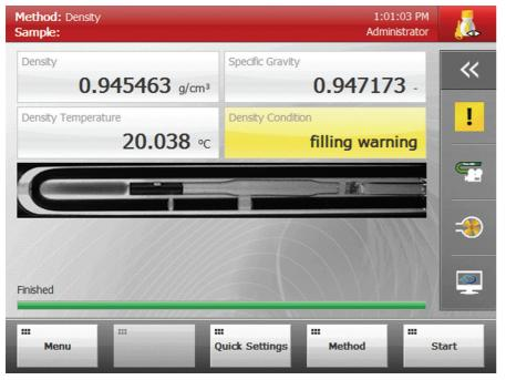
Figure 3: Screen of an "intelligent" density meter including a camera image of the U-tube and filling warning due to the bubbles in the sample
