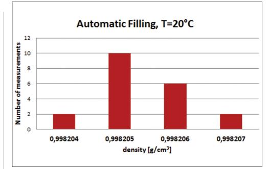
Figure 2: Automatic filling of bidistilled water at 20 °C by an autosampler (n=20; mean= 0.998205 g/cm<sup>3</sup>, STD= 8.20783E-07)
