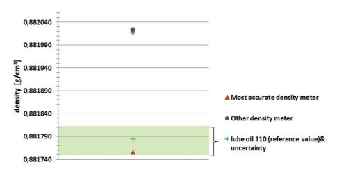
Figure 6: Deviation of measured density values of lube oil 110 (as the viscous standard reference) measured on 2 different density meter models
