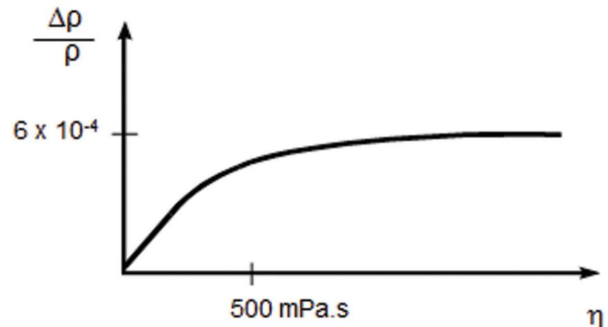
Figure 5: Viscosity influence on the density measurement based on the oscillating U-tube principle
