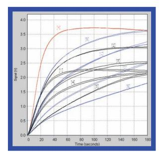
Figure 1: Measuring curves of the blanks, standards and the sample for the determination of the antioxidative capacity of the lipid soluble compounds. Voltage proportional to the generated luminescence as a function of measuring time. The inhibition (reduction) of luminescence through antioxidants in the standards [B]-[E] (0,5 1,0 2,0 und 3 nmol) (the blue lines) and the samples [1] – [5] (the black lines) compared to the blank [A] (the red lines) is to be observed.
