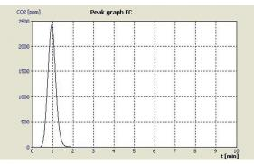
Figure 6: EC control standard, measurement curve for determining EC content
