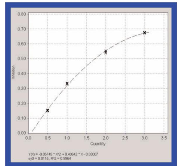
Figure 2: Calibration curve with 0,5 1,0 2,0 and 3,0 nmol Trolox® (see the corresponding measuring curves in Fig. 1)
