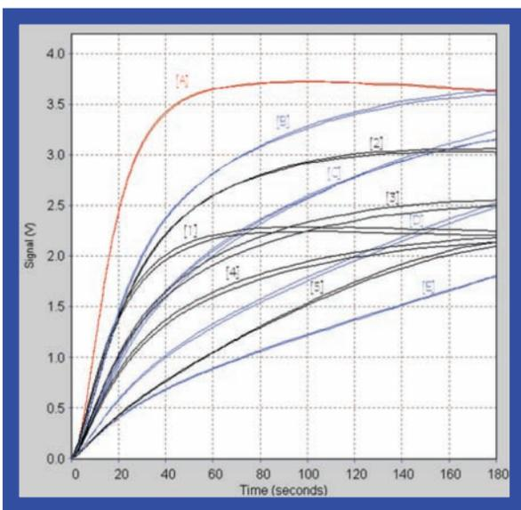
Figure 1: Measuring curves of the blanks, standards and the sample for the determination of the antioxidative capacity of the lipid soluble compounds. Voltage proportional to the generated luminescence as a function of measuring time. The inhibition (reduction) of luminescence through antioxidants in the standards [B]-[E] (0,5 1,0 2,0 und 3 nmol) (the blue lines) and the samples [1] - [5] (the black lines) compared to the blank [A] (the red lines) is to be observed.
