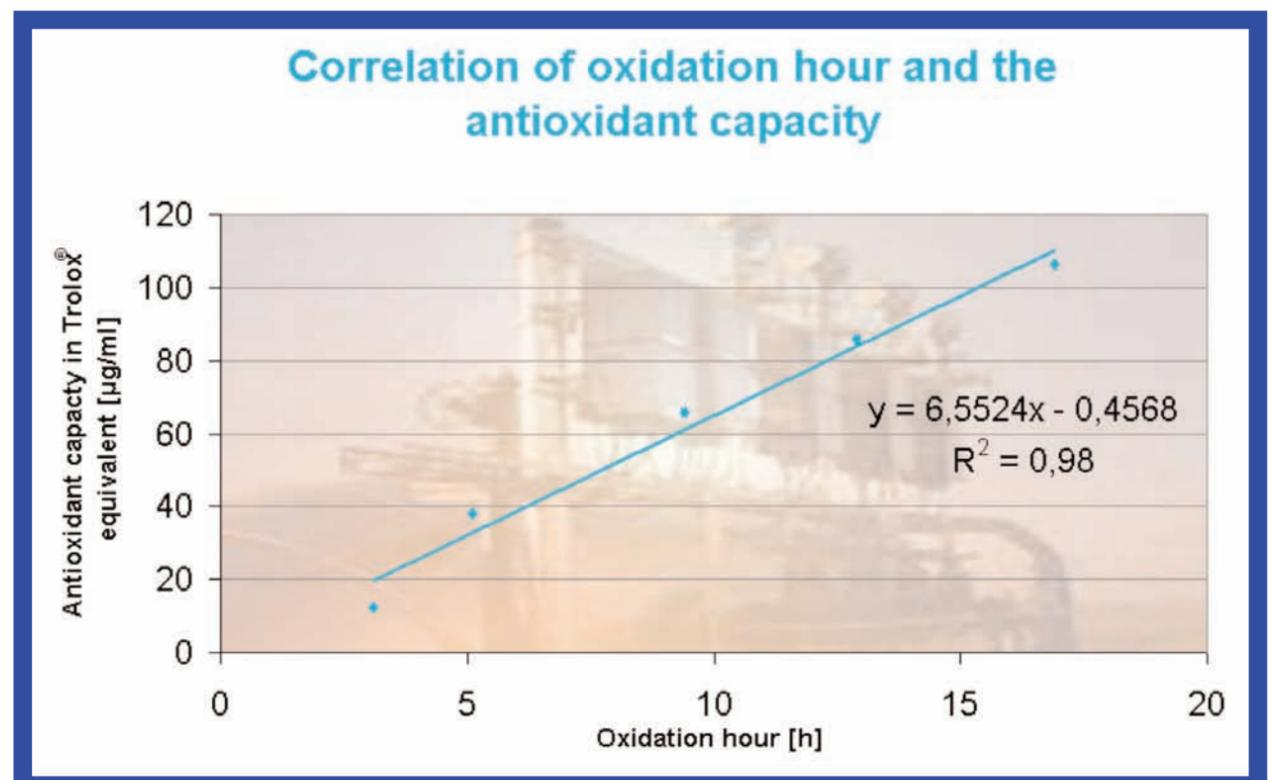
Figure 3: Correlation of oxidation hour and the antioxidant capacity in biodiesel
