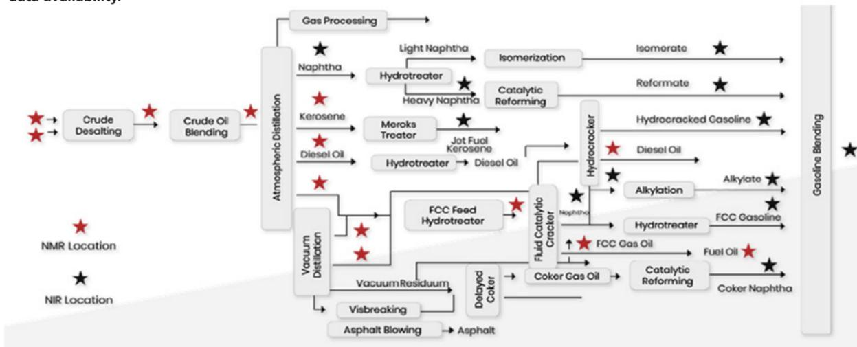
Currently, half the locations in the plant are blind spots, which are not monitored (red stars). By placing 4IR Petroleum Analysers in the red star locations, process engineers in the control room will receive online real-time data for crude oil and other opaque materials and achieve 100% coverage of all production. The red stars are unique locations where only Process NMR Analysers can provide reliable, accurate and timely measurements.
