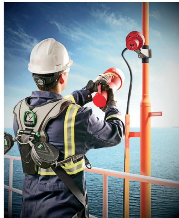
Figure 4: Flame detector being tested with TL105 test lamp
