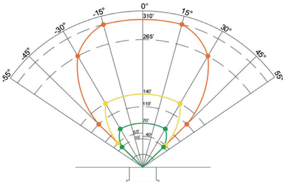
Figure 2: FL5000 Detector Extended Range & FOV Graphic
