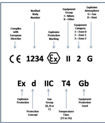
Fig. 3. Breakdown of Ex Markings
