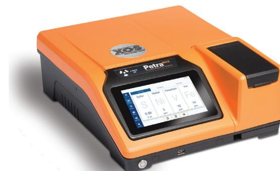
Petra MAX delivers D4294 sulfur analysis alongside rapid measurement of 12 other elements including D8252 analysis of nickel and vanadium. Petra is powered by HDXRF which delivers higher performance over traditional EDXRF.
