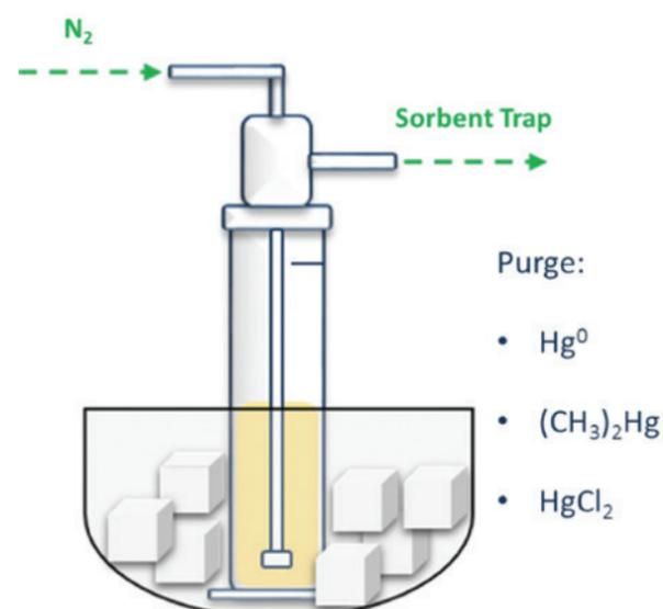
Figure 1: Schematic of purge and trap apparatus
