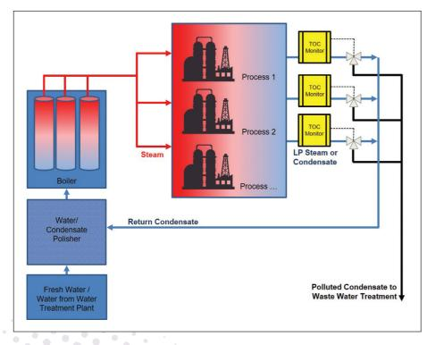
results from leakages between the product cycle and the steam cycle.
