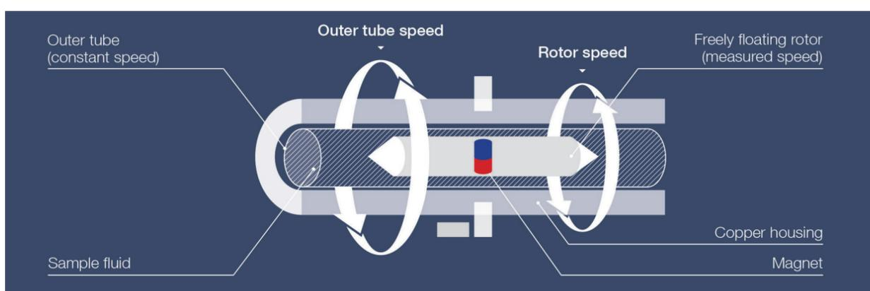
Figure 1. Stabinger Viscometer™ measuring principle
