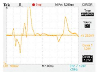
In this image, a single rod probe is measuring oil with a dielectric constant of 2. Although the desired level signal (oil surface) is evident, there are many other irregularities in the waveform baseline. Several factors can create these unwanted signals, and, if they are large enough compared to the signal amplitude, accuracy issues and/or loss of the level signal can result. With a signal of 88mV and 20 mV of noise, the SNR is:
