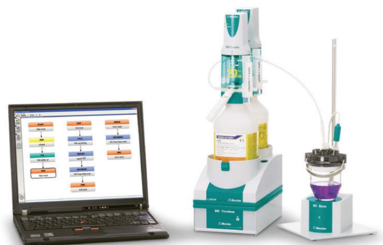
Figure 1. The 859 Tirotherm with magnetic stirrer, two Dosinos, and the tiamo™ software: This simple setup allows you to measure the acid number of crudes and refinery fractions.
