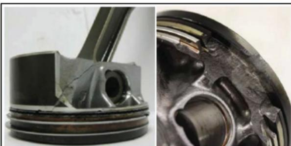
Two examples of piston damage due to LSPI
