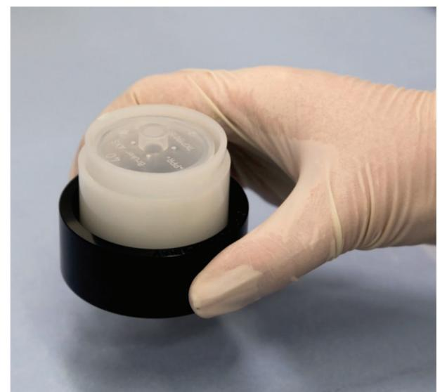
Figure 3: A preparation tool (black) is supplied for failsafe preparation of liquid cup
