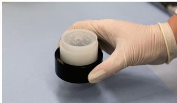
Figure 3: Liquid cup (Ø 40 mm) in SampleCare cup (Ø 51 mm). The liquid cup preparation tool can also be used to transport the sample from lab bench to measurement chamber.
