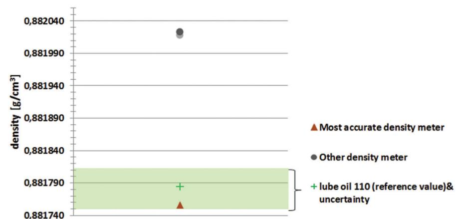
Figure 6: Deviation of measured density values of lube oil 110 (as the viscous standard reference) measured on 2 different density meter models
