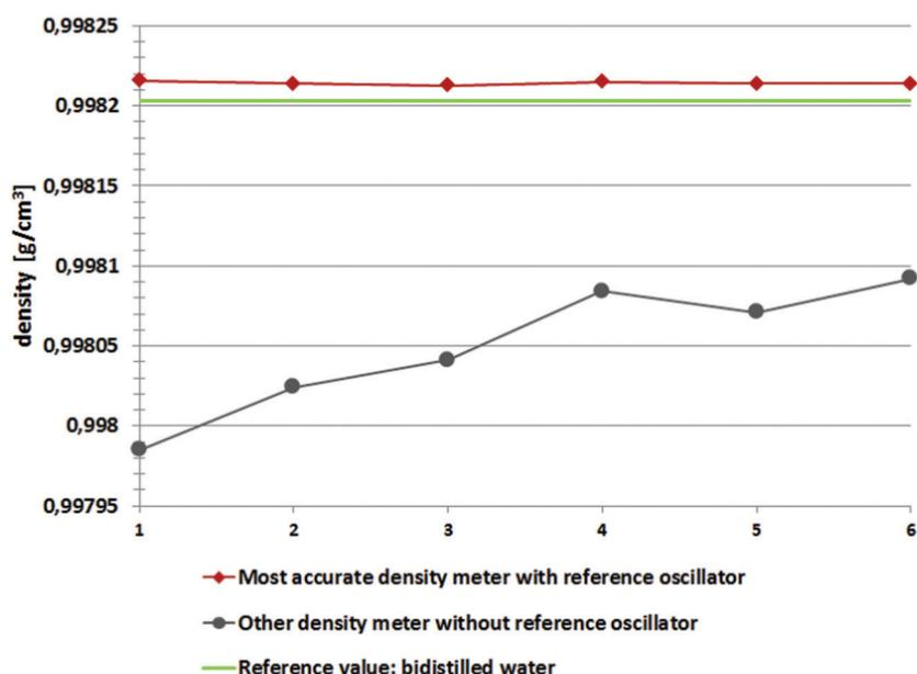
Figure 4: Density readings at 20 °C (after measurements at 80 °C) of two different density meter models, one with and one without integrated reference oscillator
