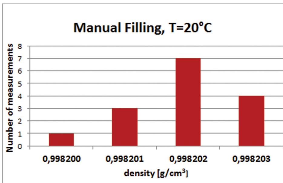
Figure 1: Manual filling of bidistilled water at 20 °C by a syringe (n=15, mean=0.99820193 g/cm³, STD= 8.8372E-07)
