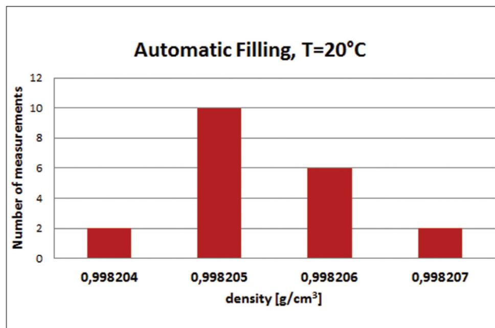
Figure 2: Automatic filling of bidistilled water at 20 °C by an autosampler (n=20; mean= 0.998205 g/cm³, STD= 8.20783E-07)
