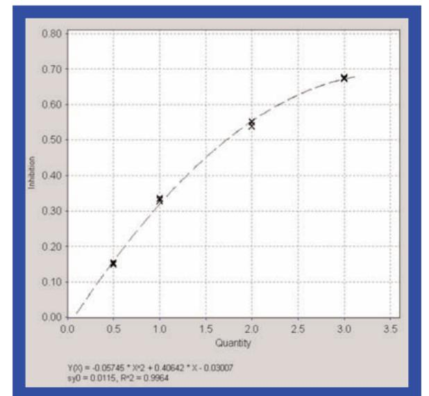
Figure 2: Calibration curve with 0,5 1,0 2,0 and 3,0 nmol Trolox® (see the corresponding measuring curves in Fig. 1)
