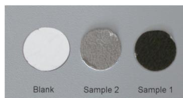
Figure 4: Filter samples for determining OC and EC content
