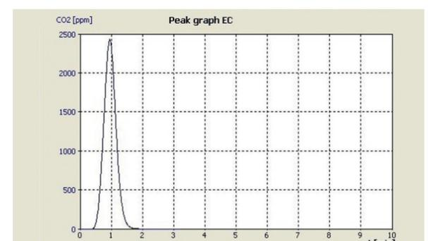
Figure 6: EC control standard, measurement curve for determining EC content
