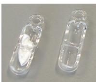
Figure 2: Special sample boat for optimal sample handling of filter samples
