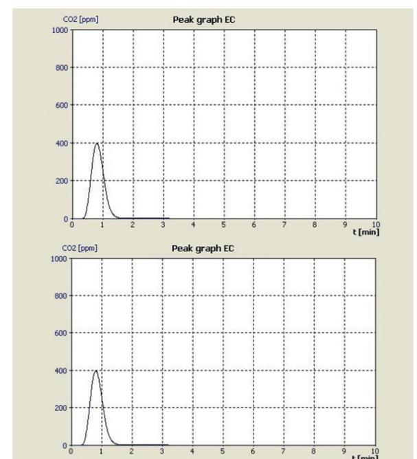
Figure 5: Filter sample no. 2, measurement curve for determining EC and OC content
