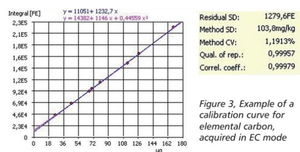
Figure 3: Example of a calibration curve for elemental carbon, acquired in EC mode
